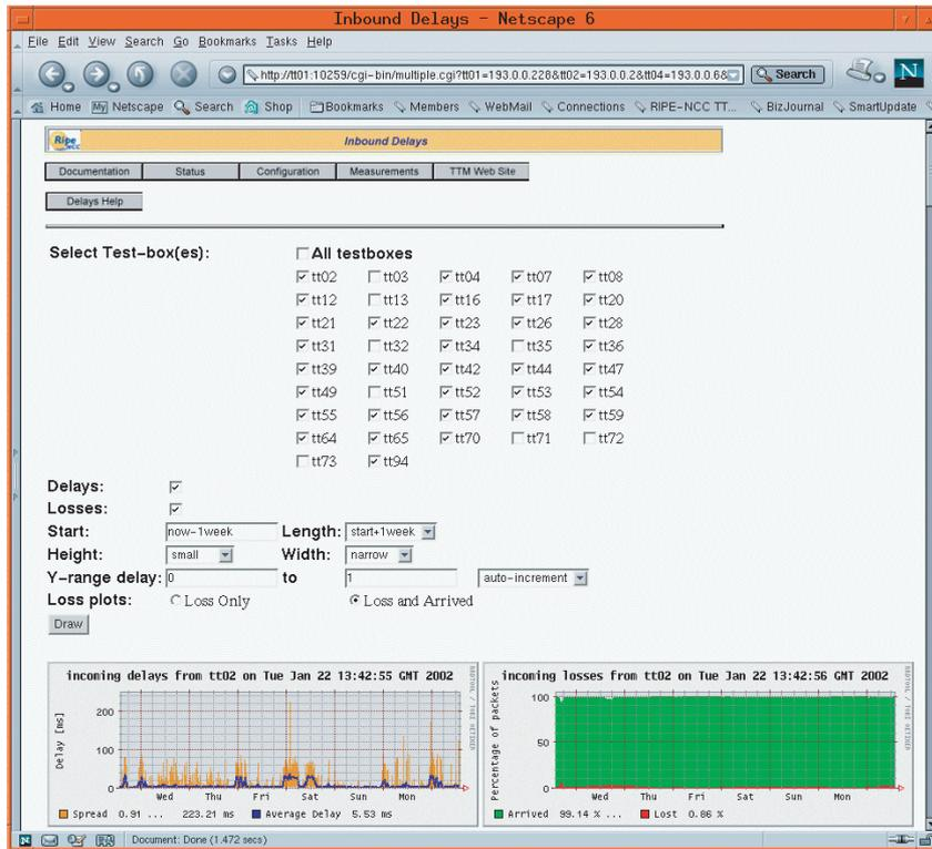
Left: Example of the web site installed on the test-boxes, showing incoming delays and packet losses.
